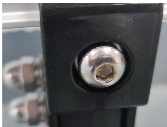
After 240 hours test - View 10
