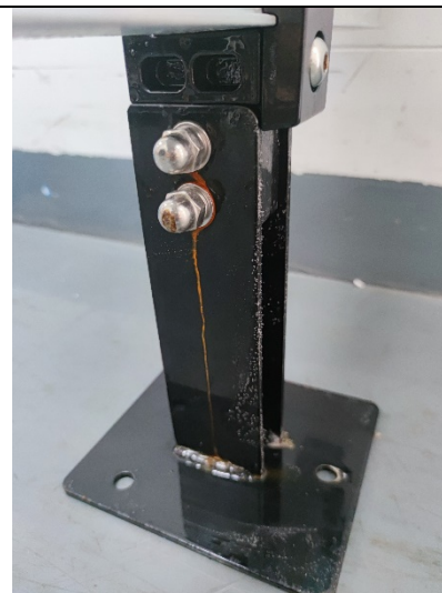
After 240 hours test - View 14
